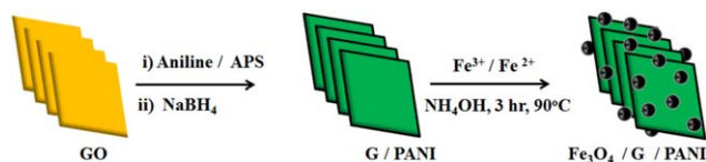
Figure 1. Synthesis of \text{Fe}_3\text{O}_4/\text{G}/\text{PANI} composite via chemical route. [Color figure can be viewed in the online issue, which is available at wileyonlinelibrary.com .]
